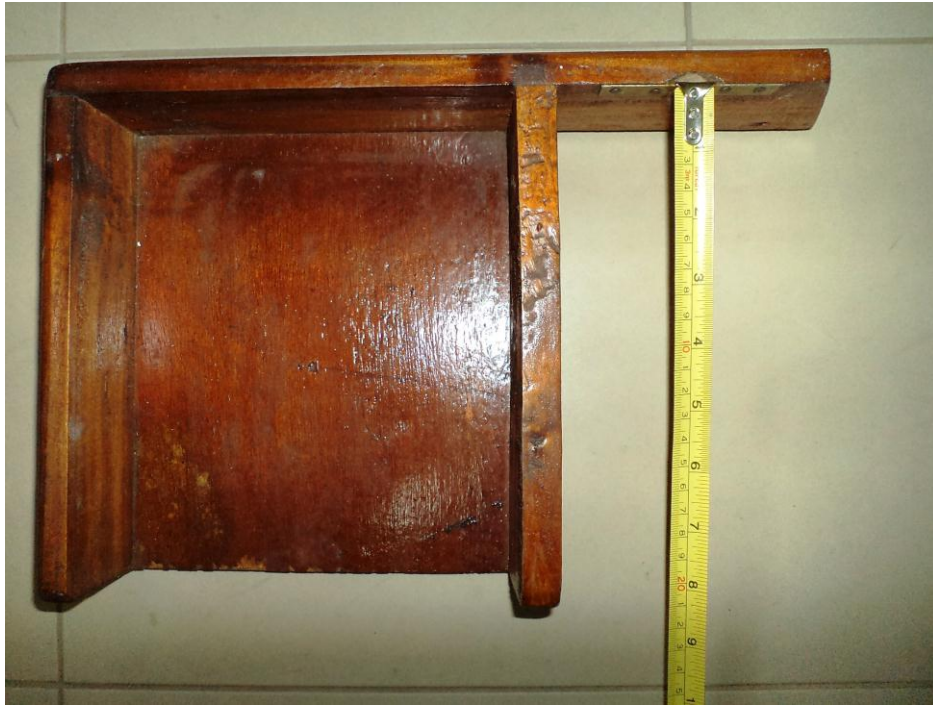
Figure 1: The device with steel measuring tape hooked on the extension arm
