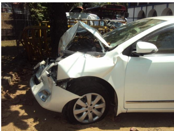
Figure 2: Extensively collapsed crumple zone.
