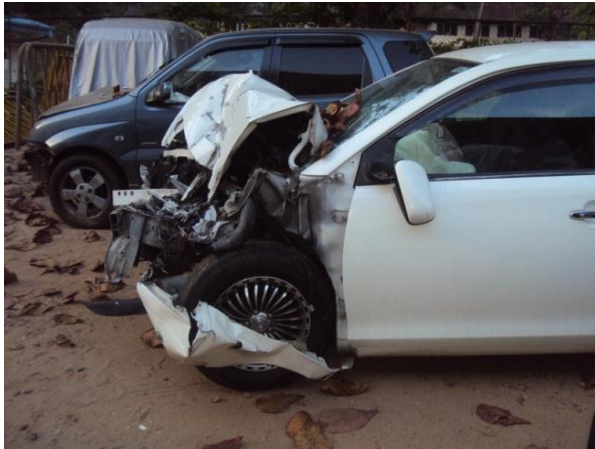
Figure 1: Extensive crumple zone damage and deployed air bags
